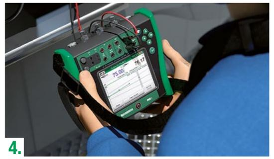
Perform calibrations/inspections in the field storing the results in a calibrator/mobile device.
