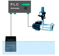
The CSC can also be connected to a ljinus level sensor LNUV3, a data logger V3 Modbus and other PLC by Modbus connection
