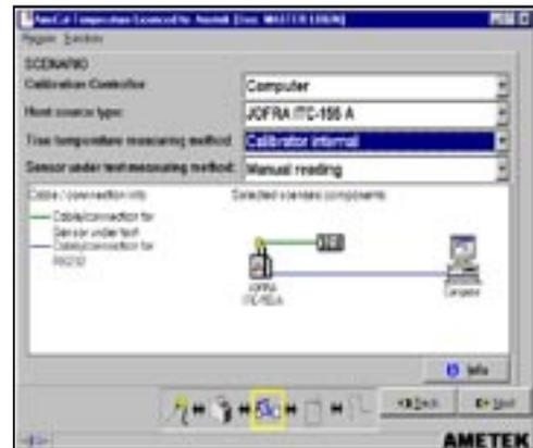
The ETC calibrator can also work with the larger AMECAL-TEMPERATURE software, which supports automatic calibration for all JOFRA dry-block calibrators equipped with an RS-232 serial data interface including the JOFRA DTI-1000 digital thermometer. For semi-automatic calibrations, the software also supports liquid baths, ice points, or other dry-block heating and cooling sources. Using the software's »SCENARIO« function allows for combining instruments in virtually any configuration.
